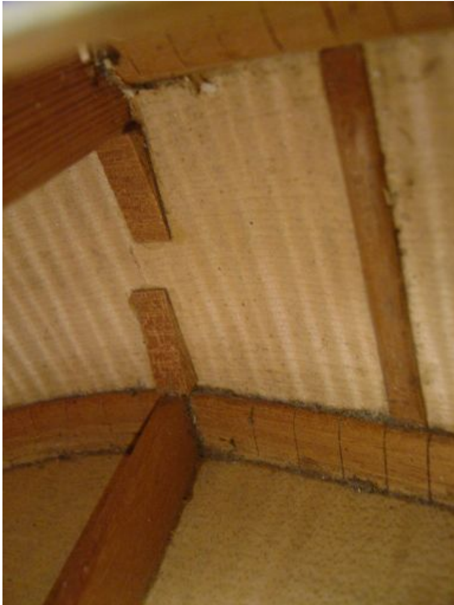
Figure A 23. Interior view of the side, kerfed lining, rib blocks, rib reinforcing bars, and transverse braces (photo courtesy James Westbrook)
