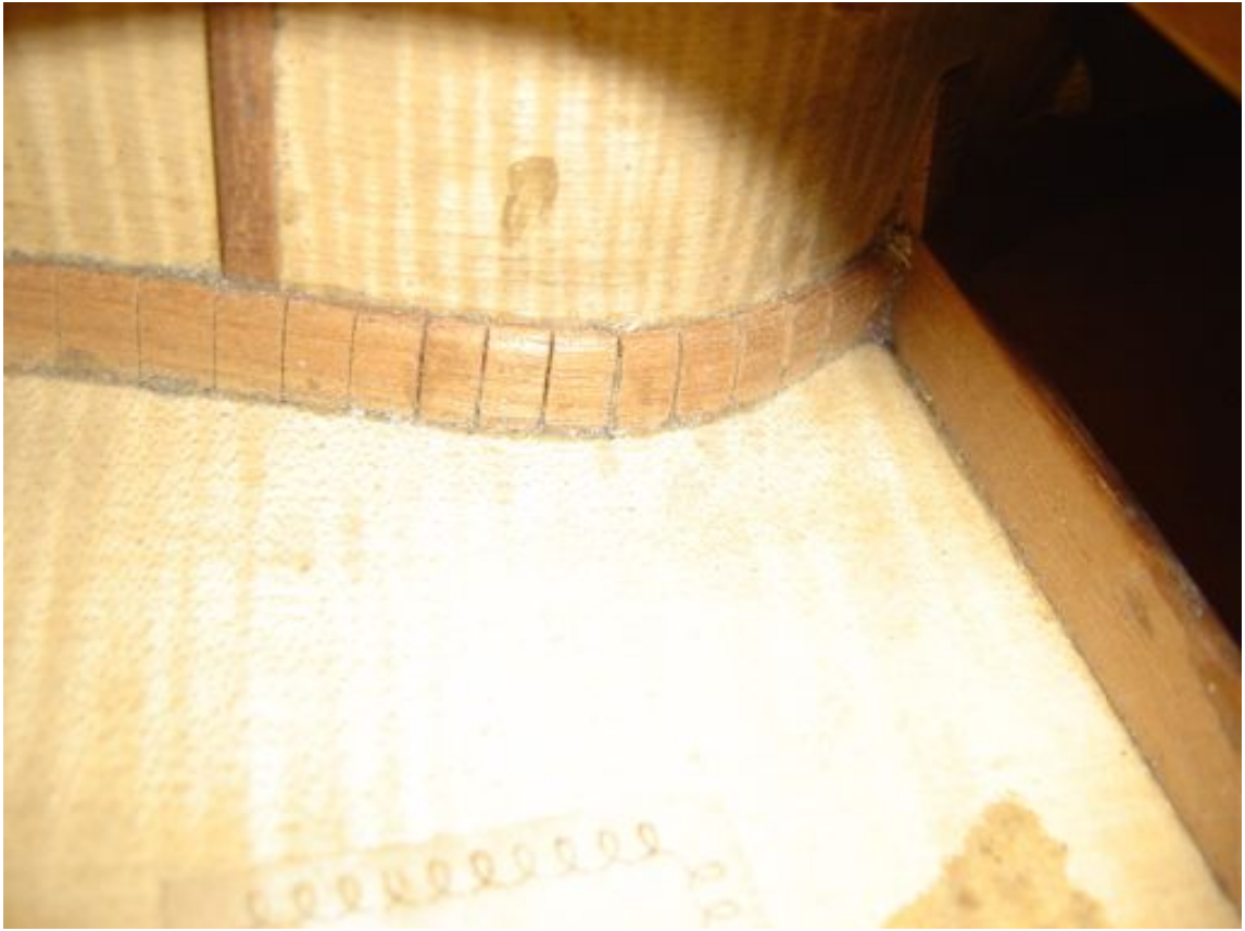
Figure A 24. Interior view of the side, kerfing and back brace (photo courtesy James Westbrook)
